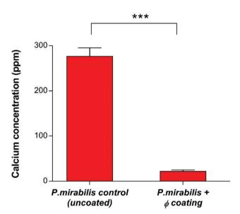
Fig. 5 Quantitative analysis of crystalline biofilm biomass on catheter surfaces by Atomic Absorption Spectroscopy (AAS). Comparison of uncoated and phage  $(\varphi)$  coated catheters 13 hours post-inoculation with *P. mirabilis*. \*\*\*P < 0.001. Data shown is the mean of triplicate repeats. Error bars represent standard error of the mean (SEM).
