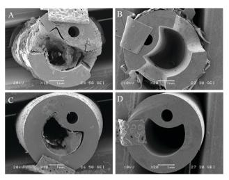
Fig. 4 SEM visualisation of catheter cross-sections comparing levels of encrustation and blockage by P. mirabilis. (A and C) Uncoated control. (B and D) With dual-layered bacteriophage coating. All catheters were removed from in vitro bladder models 13 hours after model start. (A and B) Show cross sections of catheter eyeholes. (C and D) Show cross sections of catheter lumen 1 cm below retention balloon.
