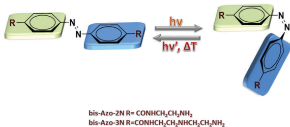
Fig. 1 Structures and interconversion pathways of the photosensitive polyamines bis-Azo-2N and bis-Azo-3N in their both relevant forms: trans and cis .
