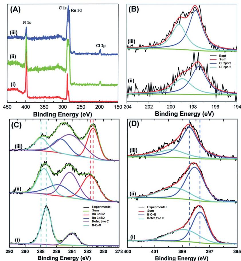
Fig. 2 (A) XPS survey spectra of (i)  $C_3N_4$ , (ii)  $C_3N_4$ -Ru-P, and (iii)  $C_3N_4$ -Ru-F. High-resolution XPS spectra of (B) Cl 2p, (C) C 1s and Ru 3d, and (D) N 1s electrons. Black curves are experimental data and colored curves are deconvolution fits.
