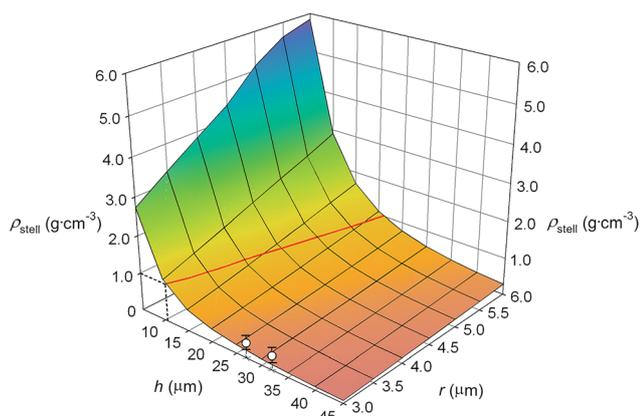
Fig. 4 Relative density  $\rho_{\text{stell}}$  of stellate Ag particles as a function of core radius  $r$  and ray length (height)  $h$ . The density of the aqueous solution is shown by the red line. (O) experimentally measured relative density  $\rho_{\text{stell}}$  of fine-dispersed Ag powders prepared from the reaction mixtures (1) and (2).
