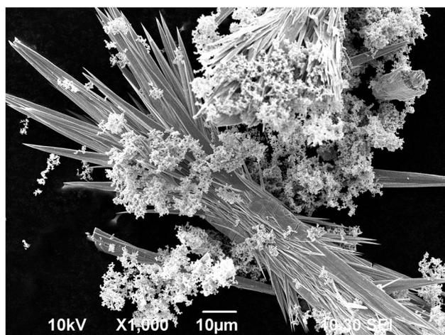
Fig. 6 SEM image of deposit from the bottom of the glass. The agglomerates resembling small blossom clusters are formed by  $\text{Ag}_2\text{S}$  nanoparticles. The long silver rays are united into compact particle bundles having a large relative density; therefore, such Ag particles do not come to the surface, but remain in the deposit.
