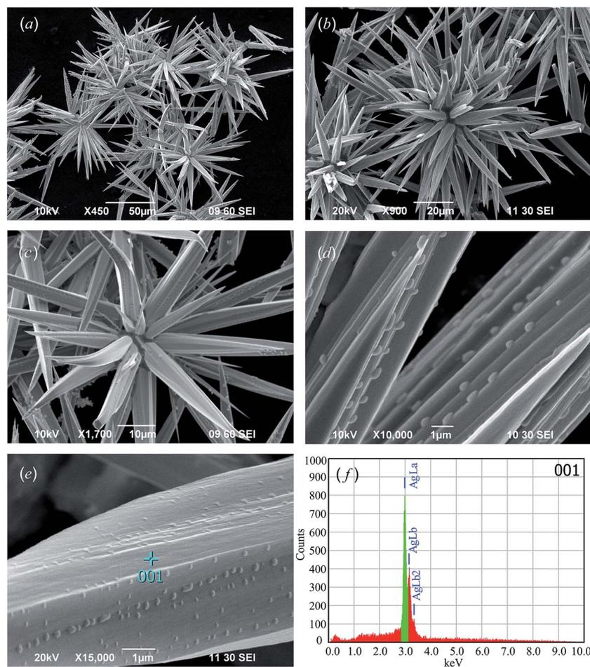
Fig. 3 The SEM images (a–c) of stellate Ag particles and (d and e) their rays. (e and f) Area on which the EDX analysis of silver particles was performed, and the results of the EDX analysis, respectively. According to the EDX data, the particles contain  $99.9 \pm 0.1$  wt% silver, *i.e.* they are metallic Ag.
