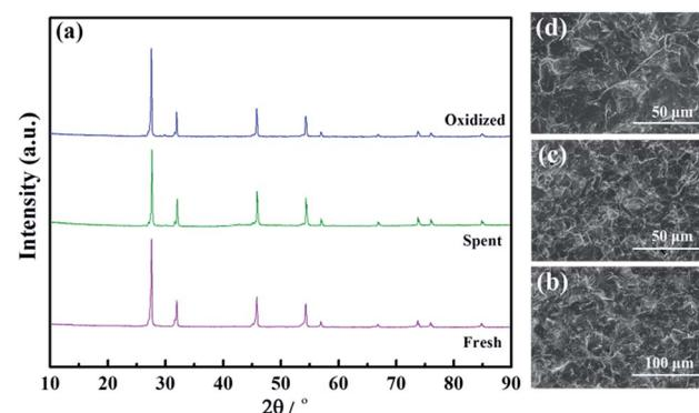
Fig. 11 The X-ray diffraction patterns (a) and SEM morphologies of fresh (b), spent (c) and oxidized (d)  $\text{La}_{5.5}\text{W}_{0.6}\text{Mo}_{0.4}\text{O}_{11.25-\delta}\text{F}_{0.05}$  membranes.
