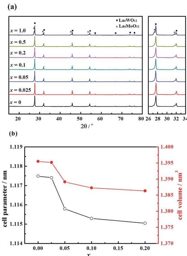
Fig. 1 (a) X-ray diffraction patterns and (b) the cell parameter and the cell volume of the  $\text{La}_{5.5}\text{W}_{0.6}\text{Mo}_{0.4}\text{O}_{11.25-\delta}\text{F}_x$  membranes sintered at 1500 °C.
