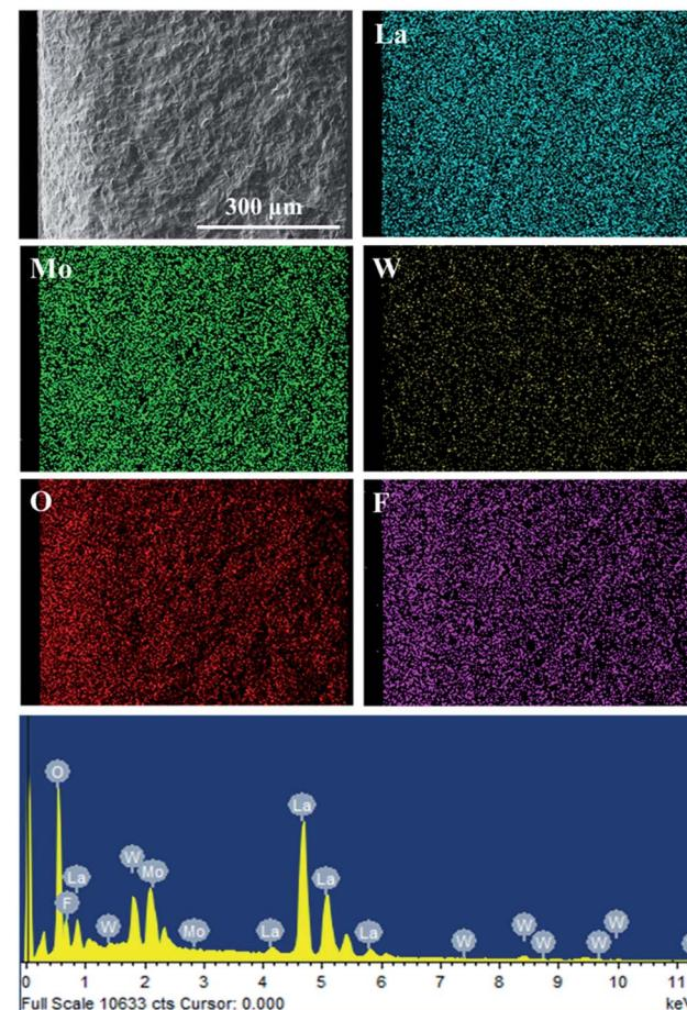
Fig. 3 SEM-EDXS image of the  $\text{La}_{5.5}\text{W}_{0.6}\text{Mo}_{0.4}\text{O}_{11.25-\delta}\text{F}_{0.05}$  membrane.
