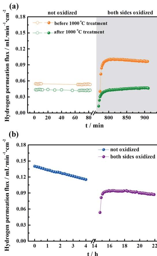
Fig. 10 (a) The regeneration of hydrogen permeation fluxes for the  $\text{La}_{5.5}\text{W}_{0.6}\text{Mo}_{0.4}\text{O}_{11.25-\delta}\text{F}_{0.05}$  membrane at 950 °C. (b) The oxidation effect on the permeability of the  $\text{La}_{5.5}\text{W}_{0.6}\text{Mo}_{0.4}\text{O}_{11.25-\delta}\text{F}_{0.05}$  membrane at 1000 °C.
