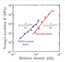
**Fig. 10** Apparent compression modulus, E, as a function of the relative density,  $\rho/\rho_{\rm s}$  of TEMPO- and Enz-CNF foams obtained by homogeneous freezing (quenching temperature of  $-68~^{\circ}{\rm C}$ ) (adapted from Martoïa  $et~al.^{32}$  Reproduced with the permission of Elsevier).
