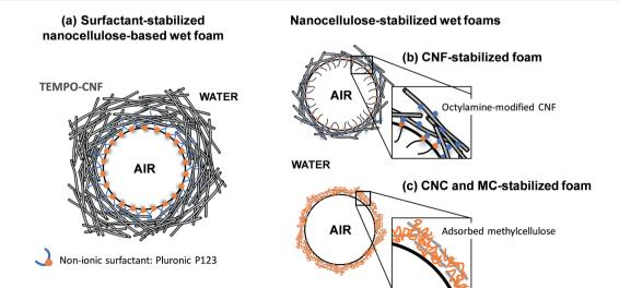
Fig. 3 Wet nanocellulose-based foams stabilized by (a) a non-ionic surfactant, 42 (b) partially hydrophobic CNF44 and (c) methylcellulose and CNC.46
