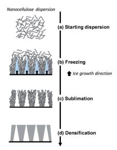
Fig. 5 Schematic diagram of directional ice-templating of nanocellulose dispersion (adapted from Deville<sup>56</sup>).
