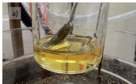
Fig. 1 (a) Liquid monosaccharide-urea melt obtained from glucose.
