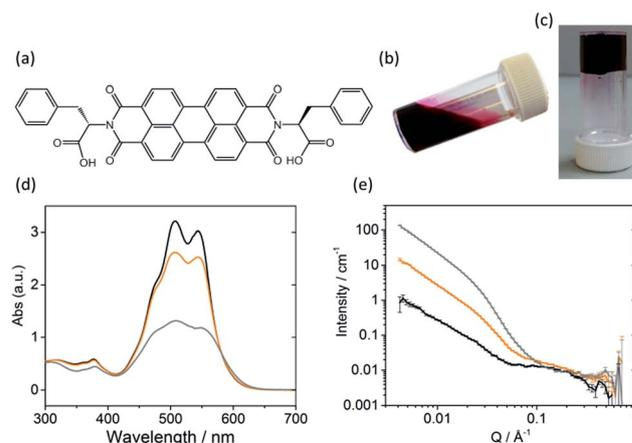
Fig. 1 (a) Molecular structure of PBI-F; (b) high pH solution (10 mg mL<sup>-1</sup> PBI-F, 2 eq. NaOH, 20 v/v% methanol); (c) low pH gel (10 mg mL<sup>-1</sup> PBI-F, 2 eq. NaOH, 8 mg mL<sup>-1</sup> GdL, 24 hours); (d) UV-Vis absorption spectra and (e) SANS data at pH 11 (black), 6 (orange), and 2 (grey). pH was lowered in (d) by HCl addition and in (e) by DCl addition.
