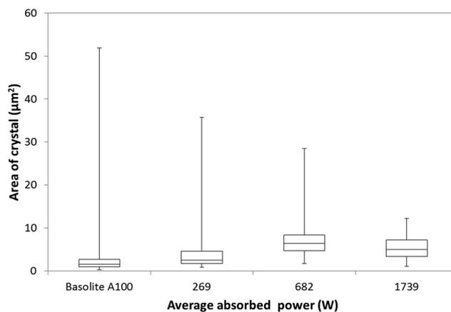
Fig. 3 Box and whisker plot of average absorbed power vs. particle size of MIL-53(Al)*ta* and commercial material Basolite A100 from SEM analyses. Error bars represent the largest and smallest particle sizes. Boxes represent the interquartile range (outer line) and median (central line) particle sizes.
