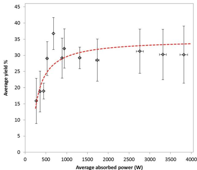
Fig. 2 Plot of average absorbed power vs. average yield of MIL-53(Al)*ta* (black diamonds) at an energy of 51  $\text{kJ mol}^{-1}$ , based on water in the reaction mixture. Predicted yield based on multiple linear regression (red dotted line, see Experimental section for further details). A microwave frequency of 2.45 GHz was used. Error bars are plotted  $\pm$  one standard deviation.
