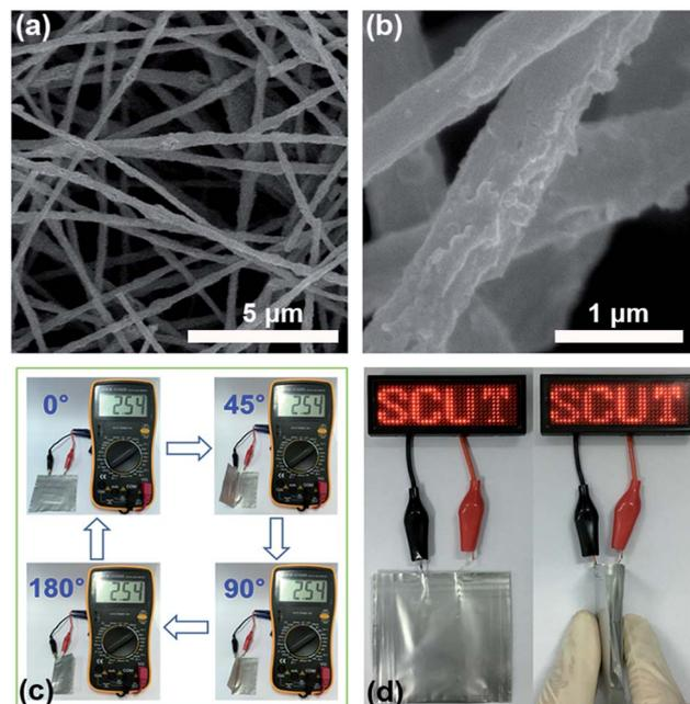
Fig. 4 (a and b) SEM images of S/G/NPCFs after 500 cycles at 5C; (c) the open-circuit voltage of a flexible battery using the S/G/NPCF electrode as the cathode at different bending angles (0–180°); (d) photographs of the LED device lit by the flexible battery during folding.
