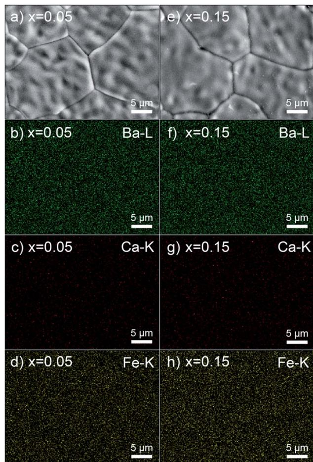
Fig. 2 Microstructure of  $\text{BaFe}_{1-x}\text{Ca}_x\text{O}_{3-\delta}$  membranes with  $x = 0.05$  (a–d) and  $0.15$  (e–h) sintered at  $1200^\circ\text{C}$  for 4 h: (a and e) SEM micrographs, (b–d, f–h) EDXS elemental distribution of Ba, Ca and Fe in panel (a and e).
