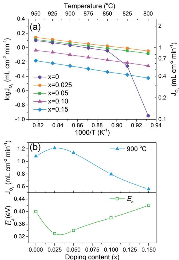
Fig. 8 (a) Temperature dependent oxygen permeation fluxes of  $\text{BaFe}_{1-x}\text{Ca}_x\text{O}_{3-\delta}$  with 1.0 mm thickness ( $F_{\text{air}} = 120 \text{ mL min}^{-1}$ ,  $F_{\text{He}} = 60 \text{ mL min}^{-1}$ ); (b) variation of the calculated activation energies and oxygen permeation fluxes at 900 °C upon doping content.
