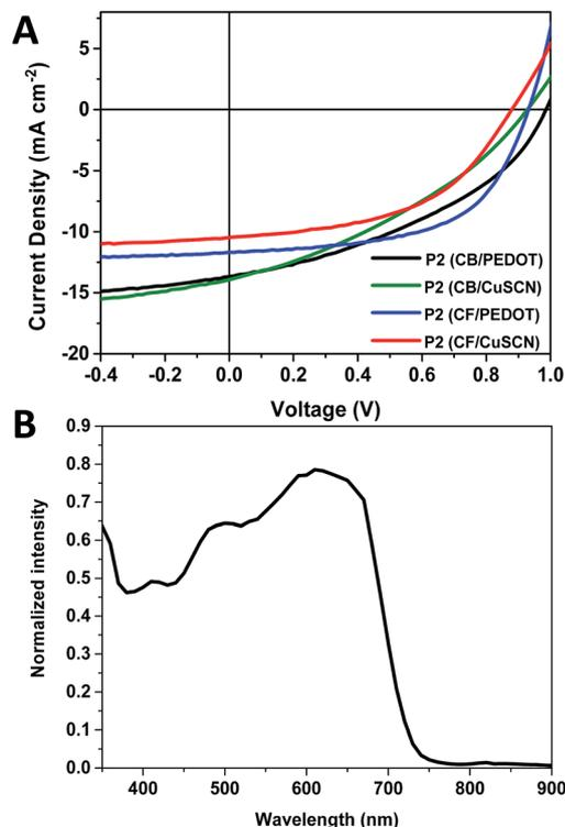
Fig. 4 (A)  $J$ - $V$  curves for either chlorobenzene (CB) or chloroform (CF) fractions of P2: PC<sub>61</sub>BM using either PEDOT:PSS or CuSCN as the hole transporting layers, (B) EQE of device made using P2 (chloroform fraction) with PEDOT:PSS as the hole transporting layer.
