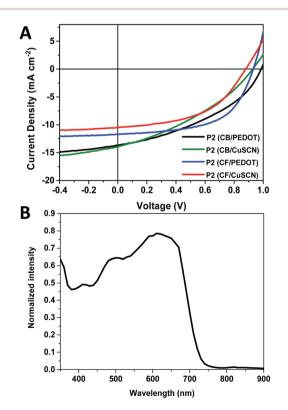
Fig. 4 (A) J-V curves for either chlorobenzene (CB) or chloroform (CF) fractions of P2:  $PC_{61}BM$  using either PEDOT:PSS or CuSCN as the hole transporting layers, (B) EQE of device made using P2 (chloroform fraction) with PEDOT:PSS as the hole transporting layer.
