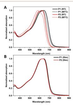
Fig. 3 (A) Absorption spectra of P1 and P2 in TCB solution and (B) P1 and P2 in thin film.
