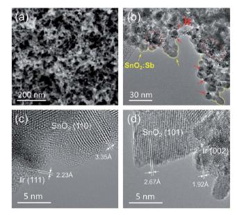
Fig. 2 (a) SEM image of  $Ir/SnO_2$ :Sb-mod-V; (b, c) 300 kV aberration-corrected HRTEM images of  $Ir/SnO_2$ :Sb-mod-V at different magnifications,  $SnO_2$ :Sb particles are lined with yellow, while Ir-containing areas are marked in red; (d) 300 kV aberration-corrected HRTEM image of  $Ir/SnO_2$ :Sb.
