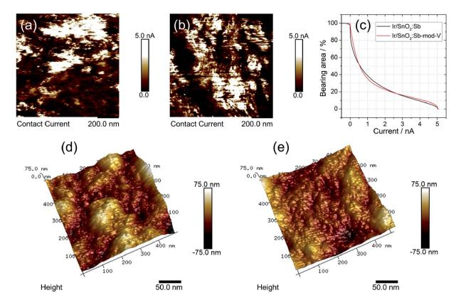
Fig. 3 AFM measurements: contact current mapping of (a) Ir/SnO<sub>2</sub>:Sb-mod-V and (b) Ir/SnO<sub>2</sub>:Sb; panel (c) shows the bearing area vs. current for the two supported catalysts, evaluated from AFM current mappings; 3D topography of (d) Ir/SnO<sub>2</sub>:Sb-mod-V and (e) Ir/SnO<sub>2</sub>:Sb.
