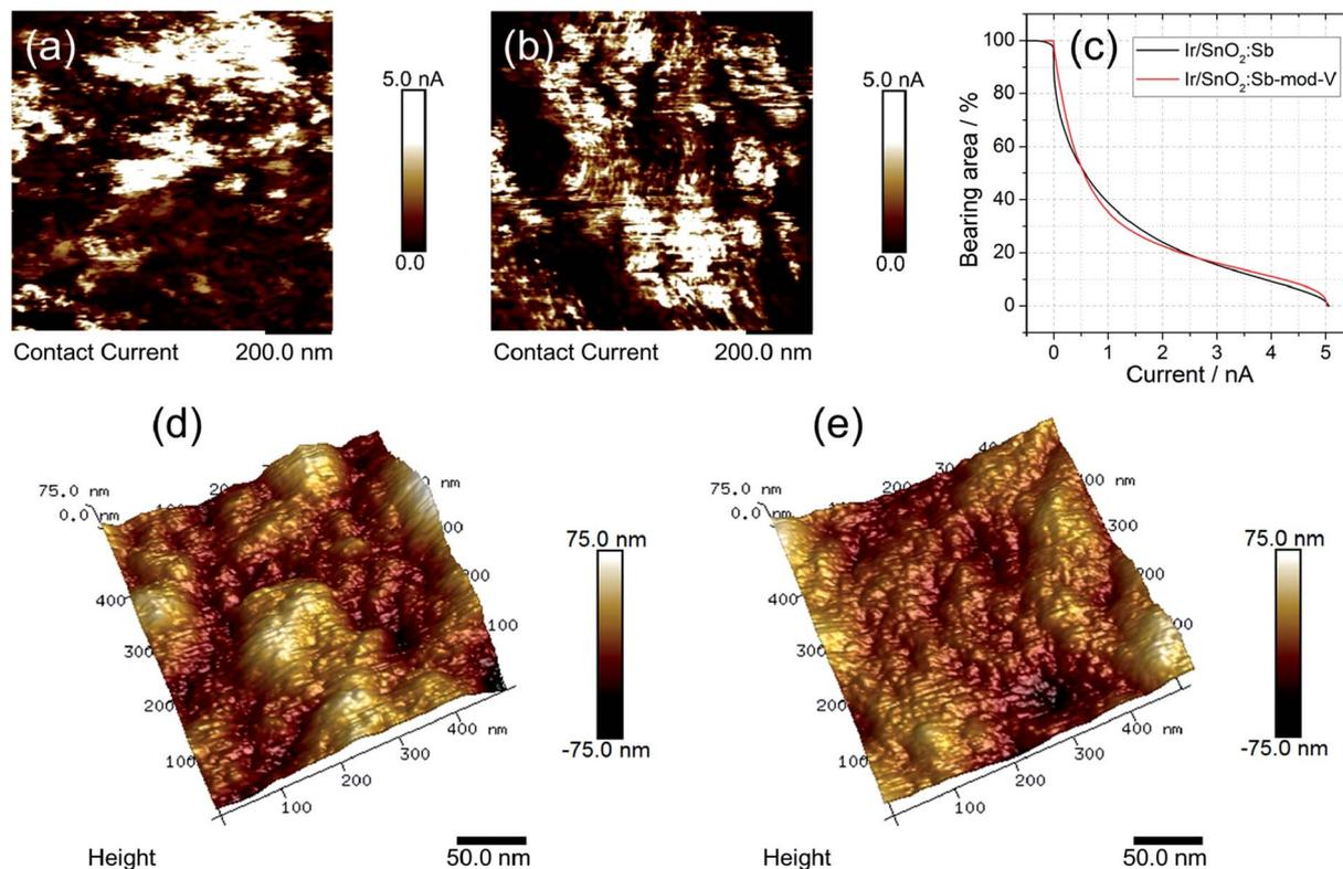
Fig. 3 AFM measurements: contact current mapping of (a) Ir/SnO<sub>2</sub>:Sb-mod-V and (b) Ir/SnO<sub>2</sub>:Sb; panel (c) shows the bearing area vs. current for the two supported catalysts, evaluated from AFM current mappings; 3D topography of (d) Ir/SnO<sub>2</sub>:Sb-mod-V and (e) Ir/SnO<sub>2</sub>:Sb.
