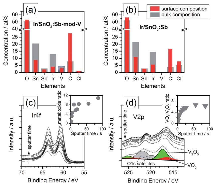
Fig. 1 XPS analysis: surface and bulk element composition profiles of (a) Ir/SnO<sub>2</sub>:Sb-mod-V and (b) Ir/SnO<sub>2</sub>:Sb. Panels (c) and (d) show detailed Ir4f and V2p spectra, respectively. In the insets of panels (c) and (d), the respective atomic ratios of Ir-metal : Ir-oxide and VO<sub>2</sub> : V<sub>2</sub>O<sub>5</sub> are plotted.
