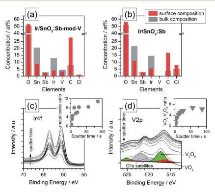
Fig. 1 XPS analysis: surface and bulk element composition profiles of (a) Ir/SnO<sub>2</sub>:Sb-mod-V and (b) Ir/SnO<sub>2</sub>:Sb. Panels (c) and (d) show detailed Ir4f and V2p spectra, respectively. In the insets of panels (c) and (d), the respective atomic ratios of Ir-metal: Ir-oxide and VO<sub>2</sub>: V<sub>2</sub>O<sub>5</sub> are plotted.
