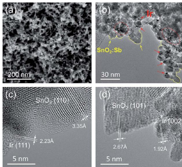
Fig. 2 (a) SEM image of Ir/SnO<sub>2</sub>:Sb-mod-V; (b, c) 300 kV aberration-corrected HRTEM images of Ir/SnO<sub>2</sub>:Sb-mod-V at different magnifications, SnO<sub>2</sub>:Sb particles are lined with yellow, while Ir-containing areas are marked in red; (d) 300 kV aberration-corrected HRTEM image of Ir/SnO<sub>2</sub>:Sb.
