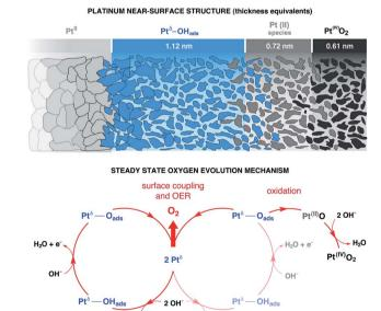
Fig. 5 Proposed catalytic mechanism and phase structure for oxygen evolution on platinum under alkaline conditions. The evaluation of the catalytic loop for oxygen evolution reaction (OER) on Pt (pH 13.9), as well as the structural description of the catalytic state, have been performed by synergistically coupling the experimental results from the operando APXPS and the corresponding numerical simulations.
