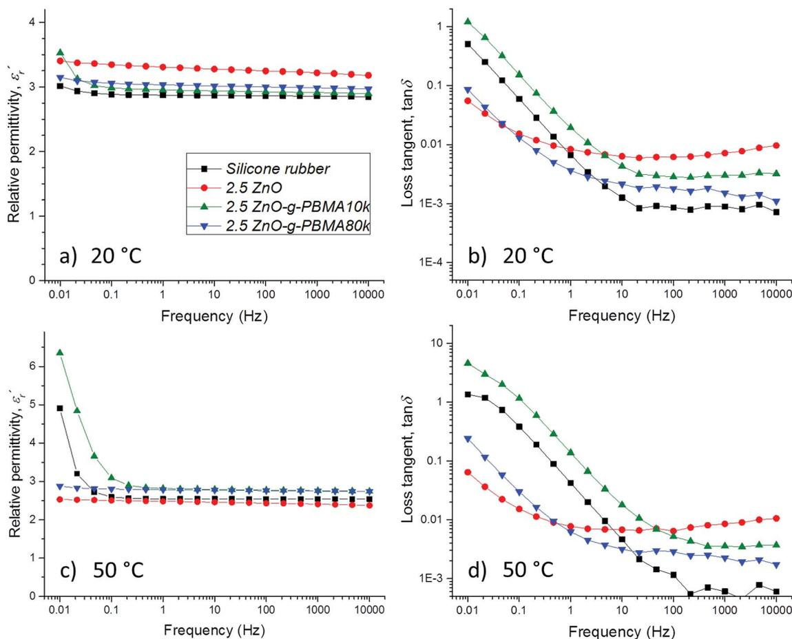
Fig. 12 Dielectric spectroscopy data of *silicone rubber*, *2.5ZnO*, *2.5ZnO-g-PBMA10k* and *2.5ZnO-g-PBMA80k* at 20 °C (a and b), and 50 °C (c and d). Fig. (a) and (c) display the relative permittivity,  $\epsilon'_r$  versus frequency, and (b) and (d) the loss tangent,  $\tan \delta$  versus frequency.
