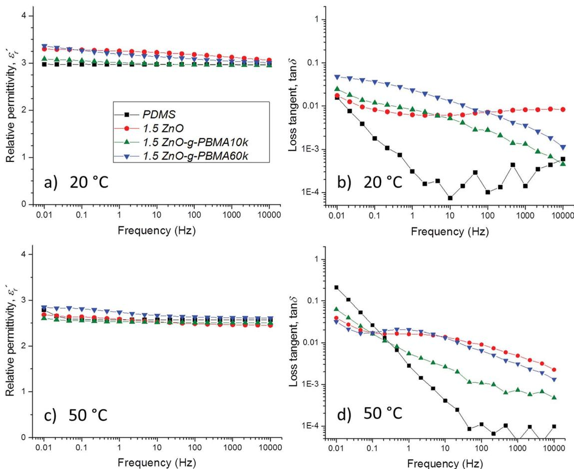
Fig. 11 Dielectric spectroscopy data of neat *PDMS*, *1.5ZnO*, *1.5ZnO-g-PBMA10k* and *1.5ZnO-g-PBMA60k* at 20 °C (a and b) and at 50 °C (c and d). Fig. (a) and (c) show the relative permittivity,  $\epsilon'_r$  versus frequency, and (b) and (d) the loss tangent,  $\tan \delta$  versus frequency.
