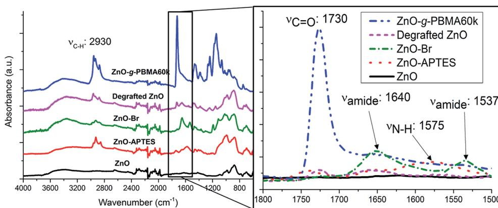
Fig. 2 FTIR spectra of ZnO, ZnO-APTES, ZnO-Br, ZnO-g-PBMA60k and degrafted ZnO between 4000 and 600  $\text{cm}^{-1}$ . Spectra have been vertically scaled and offset for clarity. The enlarged spectrum shows detailed overlapping spectra between 1800 and 1500  $\text{cm}^{-1}$  without offset.
