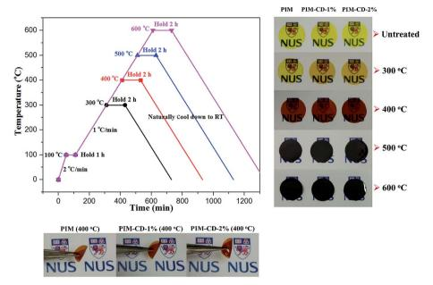
Photographs and thermal treatment procedures of PIM-CD membranes
