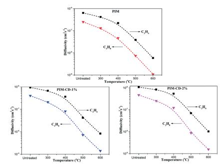
Fig. 13 The  $C_3H_6$  and  $C_3H_8$  diffusivity at 3.5 atm and 35 °C (lines are drawn to guide the eyes).
