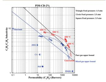
Fig. 10 Comparison of the pure and mixed gas performance of the thermally treated PIM-CD-2% membranes at 35 °C (lines are drawn to auide the eves).
