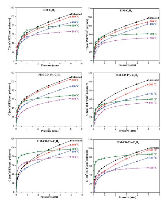
Fig. 12 Sorption isotherms of the untreated and thermally treated membranes at 35 °C.
