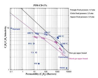
Fig. 9 Comparison of the pure and mixed gas performance of the thermally treated PIM-CD-1% membranes at 35 °C (lines are drawn to guide the eyes).
