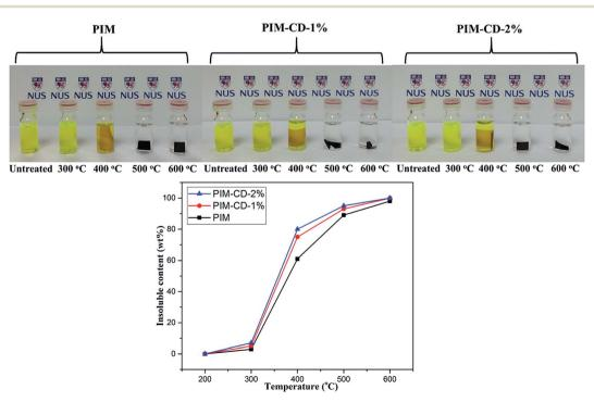
Fig. 7 The insoluble content of membranes treated at different temperatures and then soaked in DCM for 24 hours.
