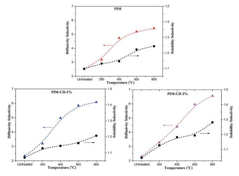
The  $C_3H_6/C_3H_8$  diffusivity and solubility selectivity at 3.5 atm and 35 °C (lines are drawn to guide the eyes)
