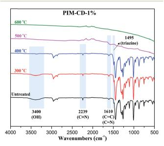
FTIR-ATR spectra of the membranes after thermal treatment.
