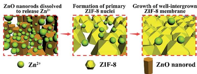
Fig. 3 Schematic illustration of proposed process for the *in situ* growth of the ZIF-8 membrane.
