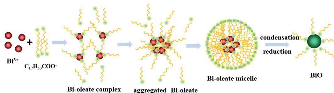
Fig. 1 Schematic illustration of the whole synthesis procedure for the BiO quantum dots.
