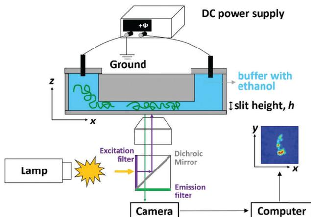
Fig. 1 Overview of our experimental system to study DNA collapse in slits. DNA molecules are driven into a nanoslit (two parallel walls with a gap in  $z$ -direction) by an electric field. The electric field is turned off once a DNA molecule enters a nanoslit. The DNA conformation projected on the  $x$ - $y$  plane ( $R_{\parallel}$ ) is recorded by fluorescent microscopy with a camera.
