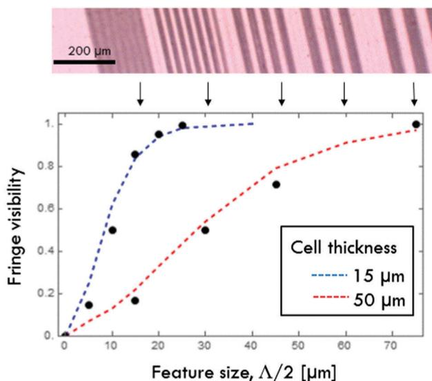
Fig. 4 Fringe visibility of a binary grating as a function of grating pitch. As predicted by a simple model (dashed lines) the measured fringe visibility (solid points) drops as the pitch approaches cell thickness. Two cases are shown: a  $15 \mu\text{m}$  thick cell with  $5 \mu\text{m}$  pixel spacing; and a  $50 \mu\text{m}$  thick cell with  $16 \mu\text{m}$  pixel spacing.
