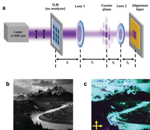
**Fig. 1** (a) Projection lithography setup. The addressable SLM is imaged onto a photoalignment surface with magnification factor  $f_2/f_1$ . The amplitude mask in the Fourier plane eliminates unwanted higher diffraction orders. (b) Grayscale input to SLM. Image: Ansel Adams, "The Tetons and the Snake River." (c) Resulting pattern in  $1 \text{ cm}^2$  area of a liquid crystal cell, viewed through crossed polarizers ( $15 \mu\text{m}$  cell thickness, filled with RM82).
