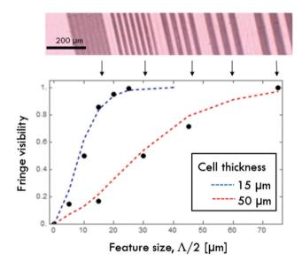
Fig. 4 Fringe visibility of a binary grating as a function of grating pitch. As predicted by a simple model (dashed lines) the measured fringe visibility (solid points) drops as the pitch approaches cell thickness. Two cases are shown: a 15  $\mu$ m thick cell with 5  $\mu$ m pixel spacing; and a 50  $\mu$ m thick cell with 16 µm pixel spacing.
