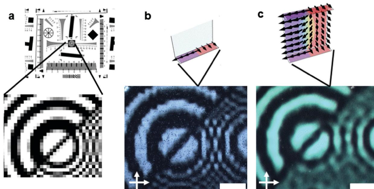
Fig. 5 Recorded test pattern to elucidate the voxel resolution limit. (a) ISO standard test pattern as displayed on the SLM. (b) Pattern as recorded at alignment surface, visualized with a spin-coated submicron layer of poly(RM257). Close agreement to the input pattern is apparent. (c) The resulting pattern templated through the thickness of a 15  $\mu\text{m}$  cell filled with RM82. Pixel edges are smoothed out by the orientational relaxation of the material. Scale bars 100  $\mu\text{m}$ .
