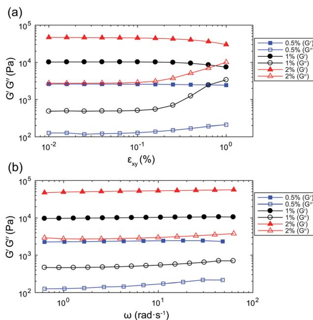
**Fig. 2** (a) Amplitude sweep for 0.5%, 1% and 2% gels, measured for shear strain amplitudes  $\varepsilon_{xy} = 0.01\text{--}1\%$  at  $\omega = 2\pi$  rad  $\text{s}^{-1}$ . (b) Frequency sweep for 0.5%, 1% and 2% gels, measured for  $\omega = (0.1\text{--}1)2\pi$  rad  $\text{s}^{-1}$  at a shear strain amplitude  $\varepsilon_{xy} = 0.06\%$ .  $G'$  (solid symbols) is the storage modulus and  $G''$  (open symbols) is the loss modulus.
