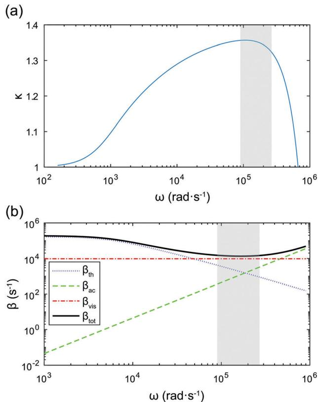
**Fig. 6** (a) Dependence of the polytropic exponent on the applied frequency. (b) Comparison of thermal, acoustic, and viscous damping coefficients as a function of frequency. The shaded areas mark the frequency range used in our experiments. The bubble radius is  $R_0 = 160 \mu\text{m}$  and  $p_0 = 1 \times 10^5 \text{ Pa}$ ,  $\gamma = 1.4$ ,  $\sigma = 67.6 \times 10^{-3} \text{ N m}^{-1}$ . Other physical properties used for the calculation are given in Table 3.
