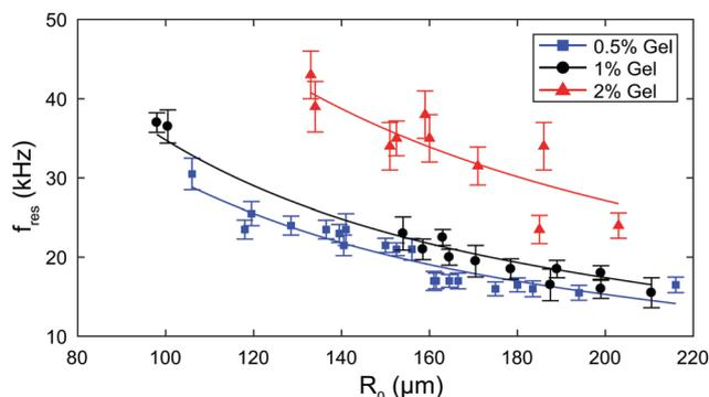
**Fig. 5** Summary of experimental data for all bubbles: resonance frequency as a function of bubble radius for each gel concentration. The solid line is a fit to eqn (9).
