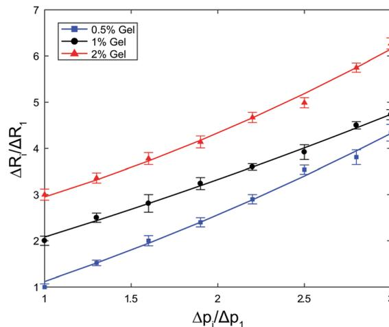
**Fig. 3** Test for linearity:  $\Delta R_i/\Delta R_1$  is the ratio of amplitudes of oscillations,  $\Delta p_i/\Delta p_1$  is the ratio of forcing amplitudes. The 1% and 2% gels are offset by 1 and 2, respectively.
