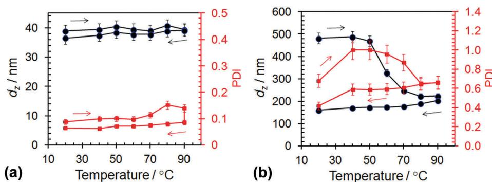
Fig. 4 Variable-temperature DLS data for dispersions of (a)  $L_{14}\text{-B}_{34}$  spheres and (b)  $L_{14}\text{-B}_{64}$  worms. The  $z$ -average diameter is represented by black circles, while the polydispersity index is represented by red squares. The arrows indicate the directions of  $z$  temperature ramps. The initial and final temperatures were 20 °C.
