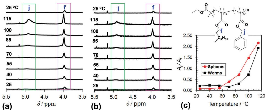
Fig. 3 Variable-temperature <sup>1</sup>H NMR spectra for dilute dispersions of (a)  $L_{14}$ -B<sub>34</sub> and (b)  $L_{14}$ -B<sub>64</sub> in dodecane-d<sub>26</sub>. The temperature was increased from 25 to 115 °C before cooling to 25 °C. (c) Signal integral ratios of j to f for the dispersions containing  $L_{14}$ -B<sub>34</sub> spheres (red circles) and  $L_{14}$ -B<sub>64</sub> worms (black squares). The changes in  $A_j/A_f$  relate to solvation changes.
