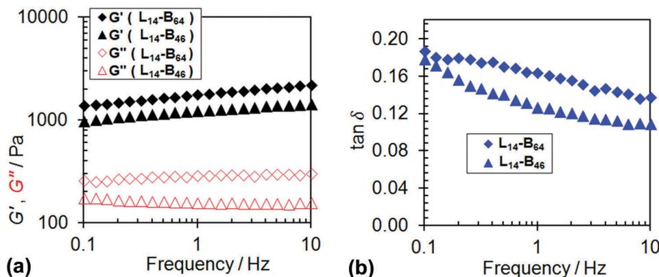
Fig. 6 (a) Dynamic frequency-sweep rheology data for the physical gels formed from  $L_{14}$ - $B_{64}$  and  $L_{14}$ - $B_{46}$  dispersed in *n*-dodecane (20% w/w). The  $G'$  (storage modulus) and  $G''$  (loss modulus) values are indicated by closed and open data points, respectively. (b) Variation of  $\tan \delta$  ( $=G''/G'$ ) with frequency for  $L_{14}$ - $B_{64}$  and  $L_{14}$ - $B_{46}$ . All data were measured at 20 °C.
