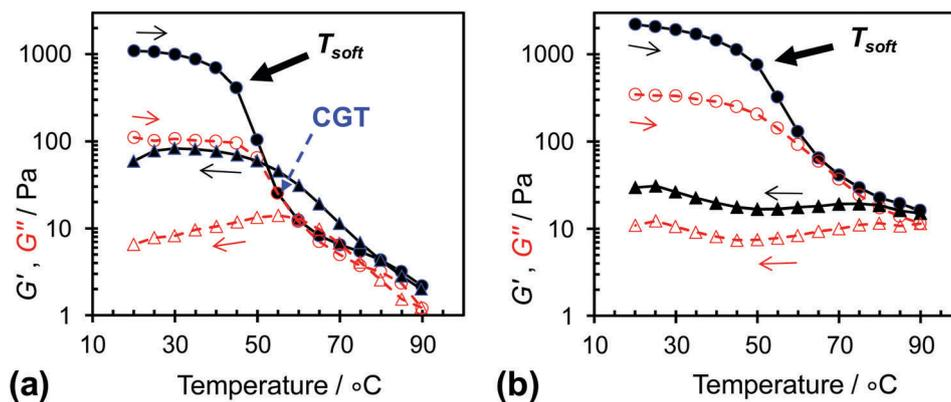
Fig. 7 Variable temperature dynamic rheological data for (a)  $L_{14}\text{-B}_{46}$  and (b)  $L_{14}\text{-B}_{64}$  dispersed in *n*-dodecane (20% w/w). The  $G'$  (storage modulus) and  $G''$  (loss modulus) values are indicated by closed data points and open data points, respectively.  $T_{\text{soft}}$  and CGT are the gel softening temperature and critical gelation temperatures, respectively (see text).
