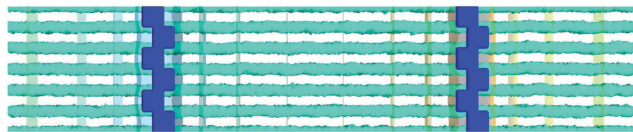
Fig. 4 Final state of the ordering on top of structured electrodes. The picture shows a view of the system from the bottom. The electrodes are shown in blue. Only the B domain with the higher dielectric constant is shown as cyan-colored stripes, the second domain is made invisible. Additional equipotential surfaces are presented to indicate the strength of the electric field in the film. The B domains register at the edges of the electrodes where the magnitude of the electric field is strongest.
