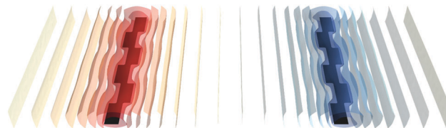
Fig. 2 System with two structured electrodes 30L_0 \times 6L_0 \times 3L_0/4 : the electrodes are shown in solid blue and red color, whereas equipotential surfaces are depicted by semi-transparent, colored surfaces. The potential values are equally spaced so that the spatial distance between equipotential surfaces is inversely proportional to the strength of the electric field, \mathbf{E} = -\nabla\psi . The structured electrodes have a periodicity L_0 in y -direction and a width L_0/2 along the x -axis. In the middle of the film between the electrodes the field is nearly homogeneous, whereas the electrode edges result in a significant enhancement of the local field.
