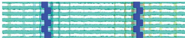
Fig. 4 Final state of the ordering on top of structured electrodes. The picture shows a view of the system from the bottom. The electrodes are shown in blue. Only the B domain with the higher dielectric constant is shown as cyan-colored stripes, the second domain is made invisible. Additional equipotential surfaces are presented to indicate the strength of the electric field in the film. The B domains register at the edges of the electrodes where the magnitude of the electric field is strongest.
