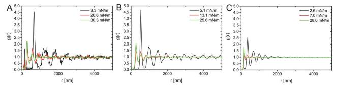
Fig. 8 Representative radial distribution functions g(r) obtained for the monolayers of the core-shell nanoparticles  $CS_{3,0}$  in (B),  $CS_{2,0}$  in (C) at different stages of compression.
