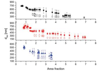
Fig. 9 Nearest-neighbour distances  $d_{NN}$  as function of area fraction for CS<sub>3.4</sub>, CS<sub>3.0</sub>, CS<sub>2.2</sub> from top to bottom. Filled symbols refer to the non-closepacked phase and empty symbols refer to the close-packed clusters.
