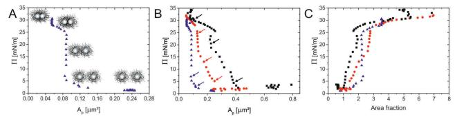
Fig. 5 Compression curves of the various CS particles: CS<sub>3.4</sub> (black), CS<sub>3.0</sub> (red) and CS<sub>2.2</sub> (blue). (A) Representation (using CS<sub>2.2</sub>) of the different interparticle interactions during compression. (B) Different compression curves of the CS particles with varying  $\lambda$ . The arrows indicate the data points corresponding to the AFM images in Fig. 7. (C) Normalised compression curves: surface pressure as a function of area fraction.
