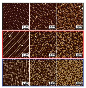
Fig. 7 AFM height images of the transferred monolayers of the core-shell particles CS<sub>3.4</sub> (black); CS<sub>3.0</sub> (red); CS<sub>2.2</sub> (blue). Increasing surface pressure from left to right. The images correspond to the data points marked by the arrows in Fig. 5B.
