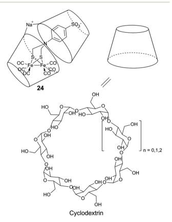
Fig. 16 Schematic representation of a diiron mimic encapsulated in a cyclodextrin unit, and the structure of the  $\alpha$  (n=0),  $\beta$  (n=1), and  $\gamma$  (n=1), a = 2) cyclodextrin units.
