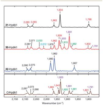
Fig. 18 FTIR spectra with normalized intensities of selected forms of semi-synthetic HydA, loaded with synthetic co-factors 30-32 (30-32-HydA1), compared to a form of HydA containing the native cofactor (CrHydA1). The figure was adapted from Berggren et al., Nature, 2013.53
