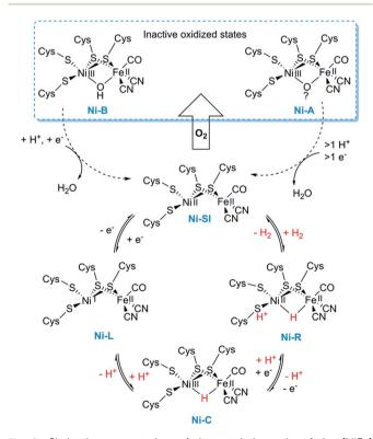
Fig. 2 Skeletal representation of the catalytic cycle of the [NiFe] hydrogenase including the Ni<sub>1</sub>-state.
