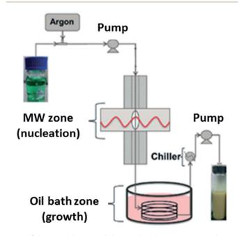
Fig. 7 Schematic diagram of the gas liquid segmented continuous flow reactor for synthesis of MOF-74(Ni) developed by Albuquerque et al.166 Reproduced from ref. 166 with permission from the Royal Society of Chemistry.
