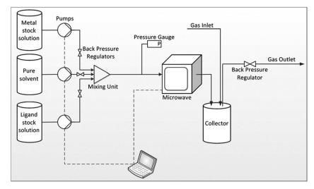
Fig. 8 Schematic diagram of the plug flow microwave reactor developed by Taddei et al. 168 Reprinted from Chemistry A European Journal, M. Taddei, D. A. Steitz, J. A. van Bokhoven, et al. Continuous-Flow Microwave Synthesis of Metal-Organic Frameworks: A Highly Efficient Method for Large-Scale Production, with permission from John Wiley and Sons. Copyright 2016 WILEY-VCH Verlag GmbH & Co. KGaA, Weinheim.
