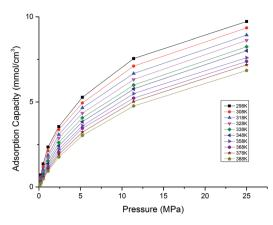
Fig. 3 Adsorption isotherms of CH<sub>4</sub> at different temperatures.
