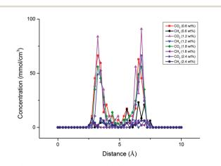
Fig. 12 Concentration profile of  $\rm CO_2/CH_4$  binary mixture adsorption in the organic shale nanopore.
