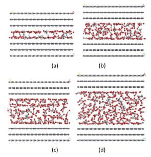
Fig. 9 Snapshots of  $CO_2/CH_4$  binary mixture adsorption for nanopores with different pore sizes: (a) 1 nm; (b) 1.5 nm; (c) 2 nm; (d) 2.5 nm.
