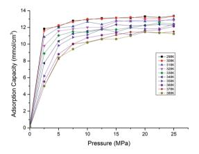
Fig. 4 Adsorption isotherms of CO<sub>2</sub> at different temperatures
