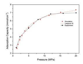
Fig. 2 Comparison of adsorption isotherms from simulation and experiment at  $333.15 \, \mathrm{K}$ .
