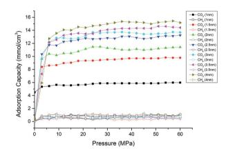
Fig. 10 Competitive adsorption isotherms of  $\rm CO_2/CH_4$  in shale organic nanopores with different pore sizes.
