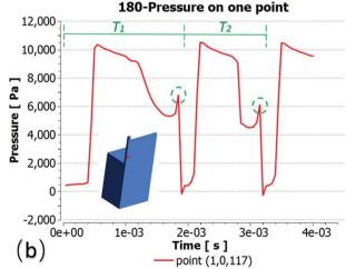
Fig. 8 Variations in pressure at one point. (a) Pressure at a contact angle of  $140^\circ$  at  $T_1=3.38$  ms. (b) Pressure at a contact angle of  $180^\circ$  at  $T_2=1.86$  ms. The point (1,0,117) was chosen to obtain a consistent droplet fracture position.
