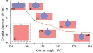
Fig. 4 Effects of the static contact angle on droplet diameter and diagrams showing terrace wetting: (I) initialization conditions for the simulation, (II)  $\theta \leq 135$ , (III)  $\theta = 140^{\circ}$ , (IV)  $\theta = 145^{\circ}$ , (V)  $\theta = 150^{\circ}$ , (VI)  $\theta = 180^{\circ}$ .
