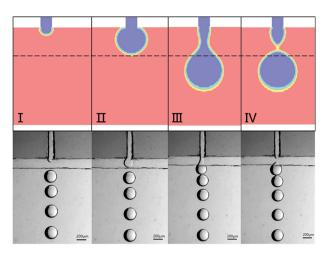
Fig. 3 A comparison of CFD simulations with experimental results. (I) Beginning of the disk expansion in the terrace. (II) The tip of the dispersed phase reaches the terrace outlet. (III) Necking occurs. (IV) Droplet detachment.
