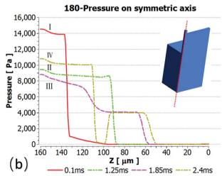
Fig. 6 The pressure along the symmetric axis indicated by the dashed line. (a) Pressure at a contact angle of  $140^\circ$  at (I) 0.08 ms, (II) 2.16 ms, (III) 3.28 ms, and (IV) 4.0 ms. (b) Pressure at a contact angle of  $180^\circ$  at (I) 0.1 ms, (II) 1.25 ms, (III) 1.85 ms, and (IV) 2.4 ms.
