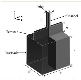
Fig. 1 A three-dimensional schematic diagram of the step model used in the current simulation.
