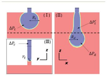
Fig. 7 Parameters used in CFD droplet simulation for step emulsification. (I) and (II) are the view from the x-z plane, and (III) is the view from the y-z plane.
