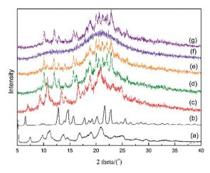
Fig. 5 PXRD patterns of solids from the suspensions after solubility determination in 0.01 M HCl medium at room temperature. (a) Initial α-Cry and (b) initial β-Cry; after solubility determination: (c) α-Cry; (d) β-Cry; (e)  $\alpha$ -AP; (f)  $\beta$ -AP and (g) CAP.
