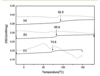
Fig. 2 TMDSC total heat flow signal (dash) and reversing heat flow signal (solid) for AZE amorphous systems: (a)  $\alpha$ -AP; (b)  $\beta$ -AP; (c)  $\alpha$ -AZE-PEZ CAP. TMDSC curves of the two APs were obtained from the data presented by Pan et al.15
