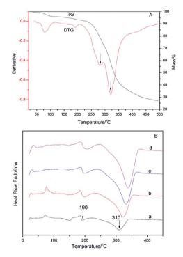
Fig. 8 (A) DTG and TG curves for the AZE-PEZ CAP ( $20 \, ^{\circ}\text{C min}^{-1}$ ) and (B) DSC curves for the AZE-PEZ CAP at different heating rates: (a)  $10 \, ^{\circ}\text{C min}^{-1}$ ; (b)  $20 \, ^{\circ}\text{C min}^{-1}$ ; (c)  $30 \, ^{\circ}\text{C min}^{-1}$ ; (d)  $40 \, ^{\circ}\text{C min}^{-1}$ .
