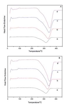
Fig. 7 DSC curves for the  $\alpha$ -AP (A) and  $\beta$ -AP (B) systems at different heating rates: (a) 10 °C min<sup>-1</sup>; (b) 20 °C min<sup>-1</sup>; (c) 30 °C min<sup>-1</sup>; (d) 40 °C min<sup>-1</sup>.
