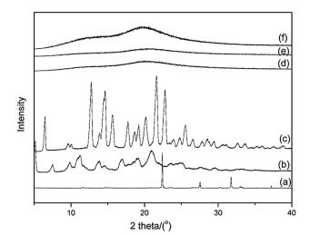
Fig. 1 PXRD patterns of the crystalline and amorphous phases of AZE. (a) PEZ; (b)  $\alpha$ -Cry; (c)  $\beta$ -Cry; (d)  $\alpha$ -AP; (e)  $\beta$ -AP; (f)  $\alpha$ -AZE-PEZ CAP.
