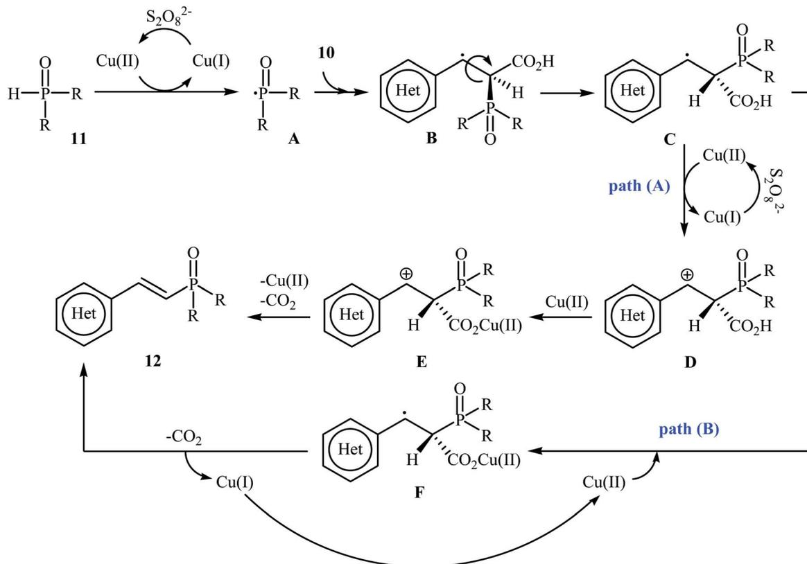
Scheme 5 Mechanistic proposal for the reactions in Scheme 4.
