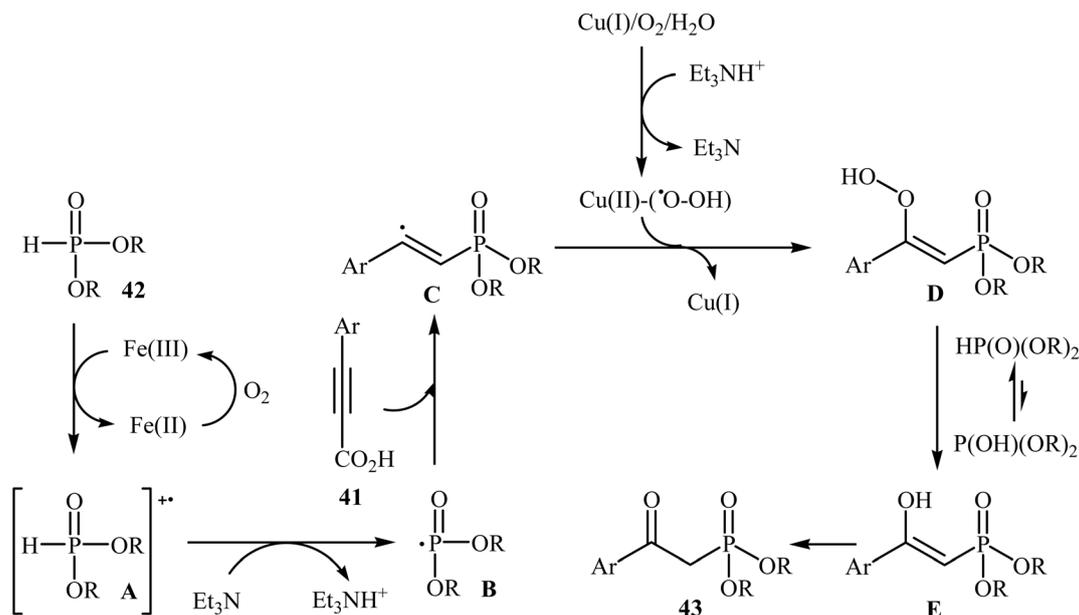
Scheme 23 Mechanistic proposal for the reaction in Scheme 22.
