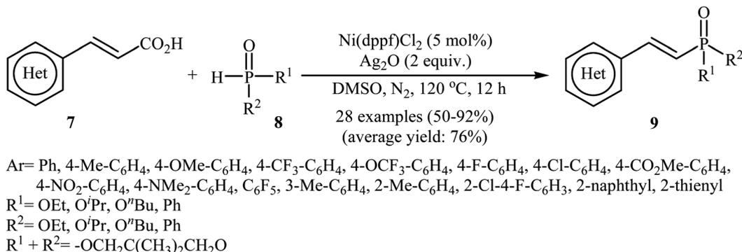
Scheme 3 Ni-catalyzed decarboxylative coupling of alkenyl acids **7** with P(O)-H compounds **8**.
