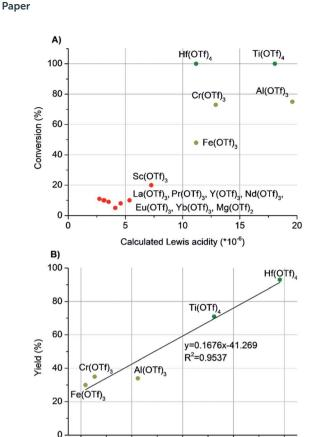
Fig. 1 (A) The conversion of 2-octanol as a function of the Lewis acidity of the metal triflate. The Lewis acidity is calculated for the metal cations, and the effect of the triflate anion is not included. (B) The yield of octenes as a function of the oxophilicity of the metal cation in the dehydration of 2-octanol. The oxophilicity is the measured M–O bond dissociation energy.<sup>21</sup>
