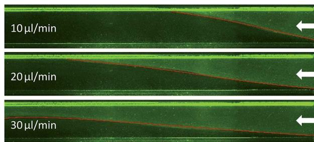
**Fig. 4** Microscopic image of the sample chamber at three different flow rates and a constant DC voltage of 100 V. The inlet is on the right side. The bright green beams are fluorescent bacteria, which were previously collected at the gel front. The red line highlights the deflection of the bacteria caused by the applied electrical field. The white arrows indicates the flow direction.
