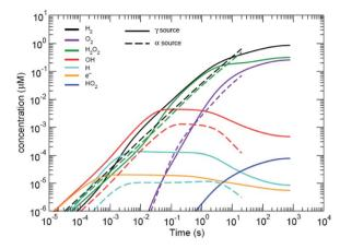
Fig. 2 Predicted radiolytic species production rates for both  $\alpha$  and  $\beta/\gamma$ radiation. The black lines corresponds to using the rate constants from ref. 15. α-Radiation results in a continuous production rate of H<sub>2</sub> and  $H_2O_2$ ; whereas, production under  $\beta$ ,  $\gamma$ -radiation reaches a steady-state condition
