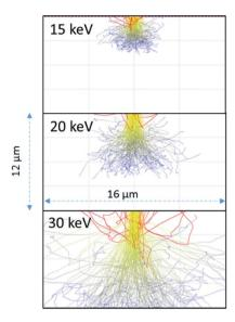
Fig. 3 Anticipated electron scattering through water for a 1  $\mu m$  wide beam at 15, 20, and 30 keV using the CASINO program.  $^{10}$  The red lines are backscattered electrons; the yellow are higher energy electrons leading to radiolytic events. The blue lines are scattered lower energy electrons although these electrons would still induce radiolytic events.
