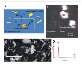
Fig. 9 (A) Schematic showing the effect of localised electron irradiation on a solution containing UO2 particles. (B) SEM-BSE image showing the formation of studtite during irradiation of UO<sub>2</sub> particles in solution. The irradiated zone is marked within the red outlined box. (C) SEM image of studtite formed from the alteration of irradiated U fuel in the K-Basins at the Hanford site, Washington, USA. (D) X-Ray energy dispersive analysis of the phase.
