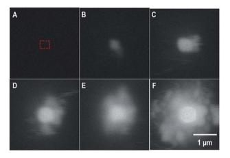
Fig. 5 SEM-BSE images from the *in situ* LC showing the formation of a uranyl peroxide over time: (A) 0 s; (B) 78 s; (C) 194 s; (D) 314 s; (E) 479 s; and (F) 640 s. The irradiation occurred over  $a < 1~\mu m^2$  region in the center.§ The blurring is the result of the fast scan to capture the image without inducing excess irradiation to the area. The dotted red box represents the region that was irradiated.
