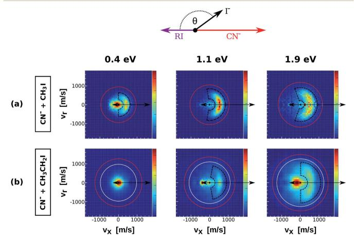
Fig. 2 Center of mass  $I^-$  velocity distributions from the reactions  $CN^- + CH_3I$  (a) and  $CN^- + CH_3CH_2I$  (b). The depicted red and white circles mark the kinematic limits for  $S_N2$  and E2 reactions. The black dashed areas represent the region of direct backward scattered events. The image for  $CN^- + CH_3I$  at 1.1 eV has been presented in a recent publication.<sup>38</sup>
