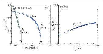
Fig. 5 Temperature variation of the antiferroelectric switching field. (a) Linear plot for [100]<sub>tetra</sub> polarization in SQA and b\*-direction polarization in [H-55dmbp][Hca] salt. Arrows indicate the antiferroelectric phase-transition temperatures. (b) Logarithmic plot for [100]<sub>tetra</sub> polarization in SQA.
