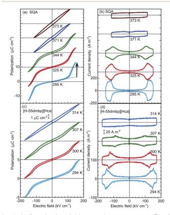
Fig. 4 Antiferroelectric switching at various temperatures. Electric polarization (P) versus electric field (E) hysteresis loops at f = 100 Hz (a, c) and corresponding current density (J) versus E (b, d) of [100]<sub>tetra</sub> polarization in SQA and b\*-direction polarization in [H-55dmbp][Hca] salt.
