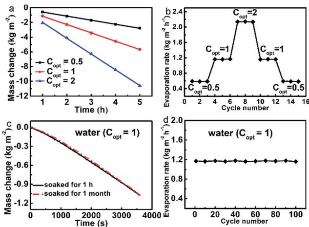
Fig. 3 Durability and stability of the evaporator. (a) The evaporation mass changes of water under different  $C_{opt}$  within 5 hours. (b) The evaporation cycle performance of the evaporator under different solar concentrations. (c) Evaporation rate curves of the evaporator soaked in water after 1 h and 1 month. (d) The evaporation cycle performance of the evaporator in water over 100 cycles, with each cycle sustained for 1 h.
