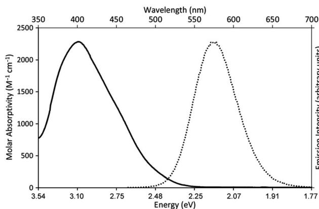
Fig. 2 UV-visible absorption spectrum of  $\text{Eu}^{\text{II}}$ 1 $\text{Cl}_2$  (—, left y-axis) and emission spectrum ( $\lambda_{\text{ex}} = 460$  nm,  $\epsilon$ :  $1044 \text{ M}^{-1} \text{ cm}^{-1}$ ) of  $\text{Eu}^{\text{II}}$ 1 $\text{Cl}_2$  (••, right y-axis). Spectra were acquired in methanol.
