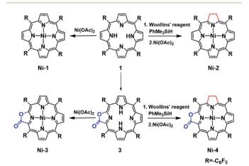
Scheme 1 The synthetic procedures for Ni-1, Ni-2, Ni-3 and Ni-4.
