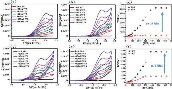
Fig. 4 Successive cyclic voltammograms of 1.0 mM Ni-1 (a), Ni-2 (b), Ni-3 (d) and Ni-4 (e) in CH<sub>3</sub>CN (0.10 M  $^n$ Bu<sub>4</sub>NPF<sub>6</sub>) at increasing concentrations of TFA from 20 mM to 140 mM. Conditions: 3 mm glassy-carbon working electrode; 25  $^{\circ}$ C; scan rate: 100 mV s<sup>-1</sup>. Graphs (c) and (f) show the TOFs vs. concentrations of TFA.
