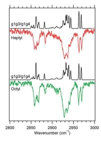
Fig. 6 Theoretical spectra of a 1:1 ratio of the g1g3 and g1g4 conformers (black) *versus* the experimental spectra of heptylbenzene (red) and octylbenzene (green) taken at 37 514 cm $^{-1}$ .
