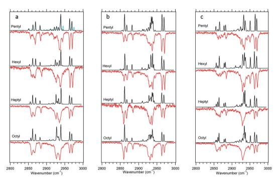
Fig. 4 (a–c) Experimental infrared spectra of pentylbenzene through octylbenzene for the all-*trans* (a), g1 (b), and g1g2 (c) conformers (red) compared to the calculated spectra for the same conformations (black). The blue spectrum on the all-*trans* pentylbenzene carries some weight from the g3 conformer (3 : 1 all-*trans* : g3 ratio).
