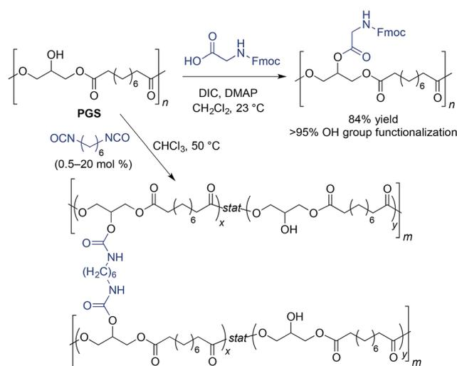
Scheme 2 Post-polymerization transformations of linear PGS: esterification with Fmoc-glycine and crosslinking with hexamethylene diisocyanate. DIC and DMAP denote *N,N*-diisopropylcarbodiimide and 4-(dimethylamino)pyridine, respectively.
