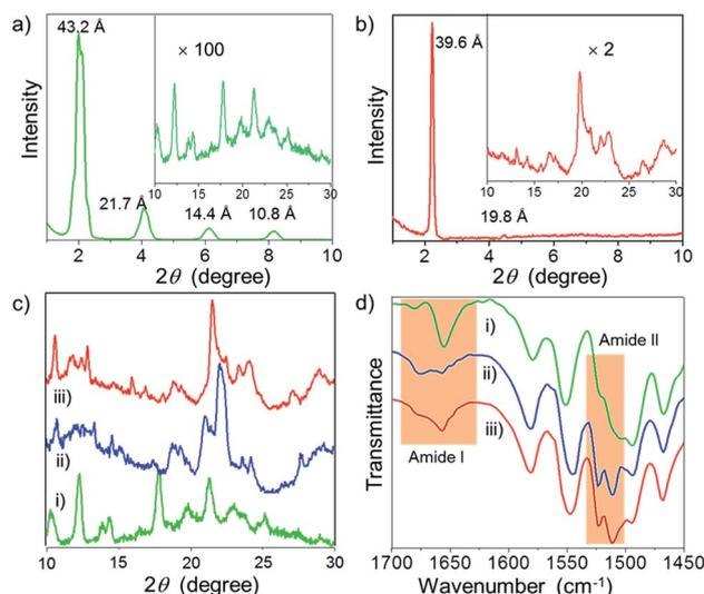
Fig. 4 WAXS of **Bodipy-1** (a) film processed from *n*-decane and (b) xerogel. (c) Comparison of WAXS ( $2\theta = 10\text{--}30^\circ$ ) and (d) FT-IR (ATR) of: (i) the *n*-decane film, (ii) the *n*-decane film after shearing and (iii) the DMSO xerogel.
