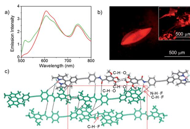
Fig. 5 (a) Emission spectrum before (red) and after (green) shearing, (b) the fluorescence microscopy image and (c) crystal packing with different interactions of the **Bodipy-2** single crystal. The inset shows the emission of the sheared crystal. The red square shows **Bodipy-2** interaction.
