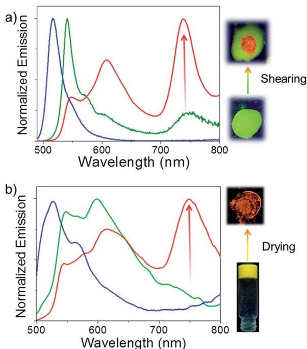
Fig. 2 (a) Emission profiles of **Bodipy-1** self-assembly in *n*-decane ( $1 \times 10^{-4}$  M, blue); film processed from *n*-decane self-assembly (green) and after shearing the film (red),  $\lambda_{\text{ex}} = 475$  nm. (b) Emission profiles of **Bodipy-1** self-assembly in DMSO solution ( $1 \times 10^{-4}$  M, blue), DMSO gel (green) and xerogel (red),  $\lambda_{\text{ex}} = 475$  nm. The corresponding fluorescence color changes under UV light illumination are also shown.
