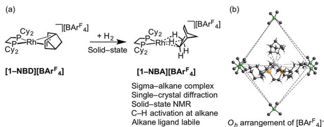
Scheme 2 (a) Synthesis of sigma-alkane complex [1-NBA][BAR<sup>F</sup><sub>4</sub>] by solid/gas reactivity; (b) O<sub>h</sub> arrangement of [BAR<sup>F</sup><sub>4</sub>]<sup>−</sup> anions in the solid-state that encapsulate cation (Ar<sup>F</sup> groups removed).
