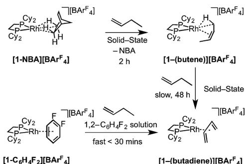
Scheme 11 Synthesis of [1-(butene)][BAR<sup>F</sup><sub>4</sub>] and [1-(butadiene)][BAR<sup>F</sup><sub>4</sub>] by solid/gas and solution routes.
