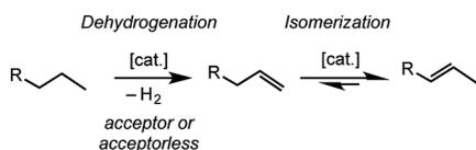
Scheme 1 Dehydrogenation/isomerization of simple, light, alkanes (R = alkyl).
