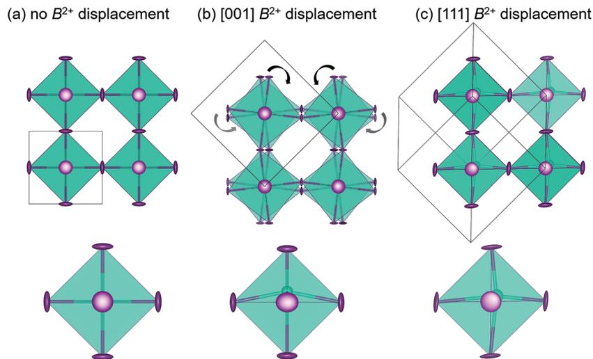
Fig. 1 Crystal structures chosen to model the X-ray PDF data: (a) cubic  $Pm\bar{3}m$  with no B-site off-centering or octahedral rotations, (b) tetragonal  $I4cm$  with allowed B-site off-centering and static octahedral rotations, and (c) rhombohedral  $R3m$  with allowed B-site off-centering and no octahedral rotations.
