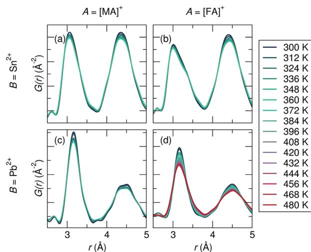
Fig. 2 Overlay of the raw X-ray PDF data collected over a range of 300 K to  $T_{\max}$  for (a)  $MASnI_3$  ( $T_{\max} = 360$  K), (b)  $FASnI_3$  ( $T_{\max} = 360$  K), (c)  $MAPbI_3$  ( $T_{\max} = 360$  K), and (d)  $FAPbI_3$  ( $T_{\max} = 480$  K). Peak asymmetry of the first B–I correlation at approximately 3 Å is observed in all compositions, but is most pronounced in the Sn compositions.
