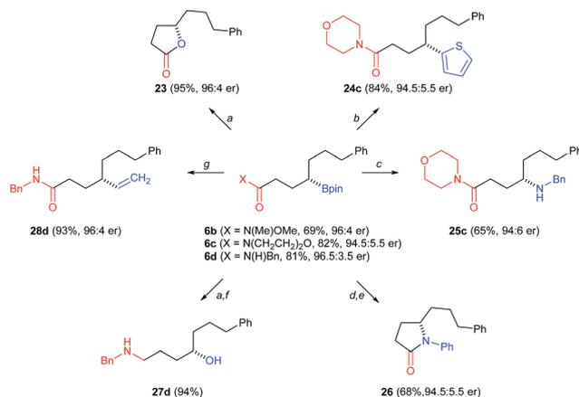
Fig. 4 Stereospecific transformations of organoboranes **6b–d**. Conditions: (a) NaOH/H<sub>2</sub>O<sub>2</sub>; (b) (i) *n*-BuLi, thiophene, (ii) NBS; (c) BCl<sub>3</sub>, BnN<sub>3</sub>; (d) BCl<sub>3</sub>, PhN<sub>3</sub>; (e) 6 M HCl; (f) LiAlH<sub>4</sub>; (g) (i) vinylMgBr, (ii) I<sub>2</sub>/NaOMe.
