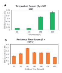
Fig. 2 MS quantitation of DPH synthesis from chlorodiphenylmethane.
