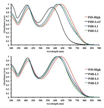
Fig. 7 UV-Vis spectra of P4S and P4H series (solution in CHCl<sub>3</sub>).
