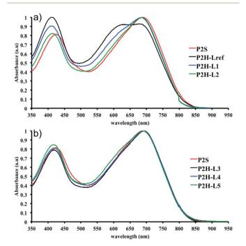
Fig. 4 UV-Vis spectra of P2S and P2H series (solution in CHCl<sub>3</sub>).
