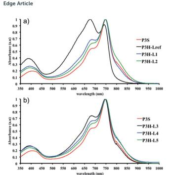
Fig. 6 UV-Vis spectra of P3S and P3H series (solution in CHCl<sub>3</sub>).
