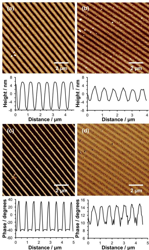
Fig. 6 (a and b) Tapping mode AFM topographical images and corresponding representative line sections obtained for nanostructured POEGMEMA brushes before (a) and after (b) *in situ* growth of PCysMA brushes within the channels between the POEGMEMA brushes. (c and d) AFM phase images acquired simultaneously with the topographical images in (a and b), together with the corresponding line sections.
