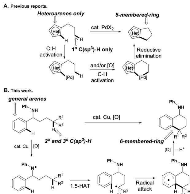
Scheme 1 Transition-metal-catalyzed intramolecular C(sp<sup>3</sup>)-H/C(sp<sup>2</sup>)-H cross-coupling.
