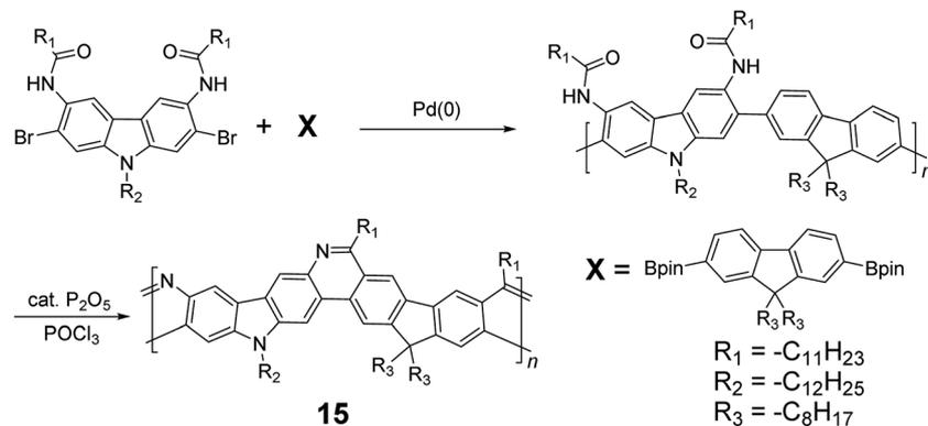
Scheme 5 Synthesis of carbazole-fluorene-based ladder polymer **15** by Bischler-Napieralski cyclization.
