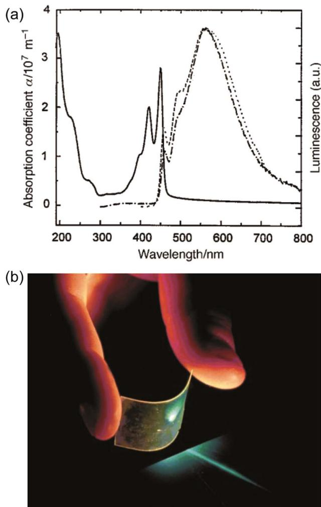
Fig. 7 Optical properties of ladder polymers. (a) Absorption (—) and PL spectra (---) of a thin film of MeLPPP **12**. (b) A photo of a blue, flexible laser made from MeLPPP **12**. Reproduced from ref. 2 with permission from The Royal Society of Chemistry.
