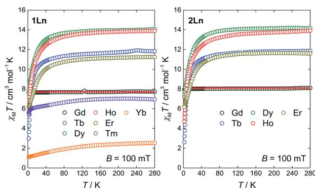
Fig. 7 Temperature dependence of the  $\chi_M T$  products for powder samples of **1Ln** (Ln = Gd–Yb, left) and **2Ln** (Ln = Gd–Er, right) recorded in a static magnetic field of  $B = 100$  mT. The red lines represent fits of the gadolinium data to an isotropic Zeeman Hamiltonian.
