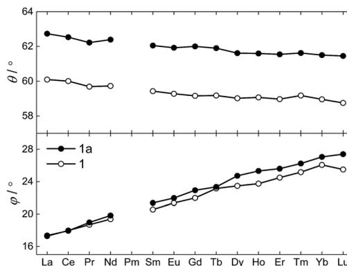
Fig. 3 The compression angle  $\theta$  (top), and the twist angle  $\varphi$  (bottom), for **1Ln** at  $T = 122(1)$  K as function of the lanthanide, determined from the X-ray single crystal structures. 1 and 1a refer to the values related to the crystal field environments defined by the O1 and O1a atoms, respectively.
